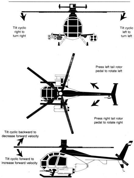
Figure 2. Helicopter Flight Control Surfaces
